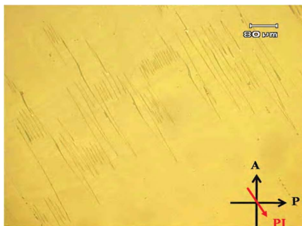
Figure 3. The SSFLC texture of the CS1024 + 1 wt% susp. at 30°C under 200 times POM magnification. (The red arrow indicates the polyimide (PI) alignment rubbing direction. Colour refers to the online version.)
